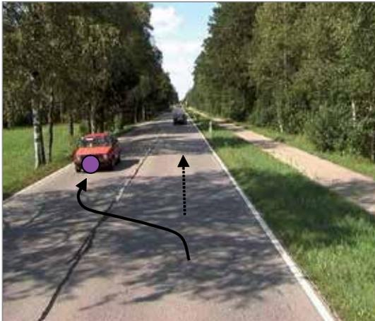
The road provided little opportunities for overtaking while the volume of traffic was quite high. Overtaking despite short time gaps in incoming traffic repeatedly caused severe accidents involving longitudinal traffic (rear-end and head-on collisions).
