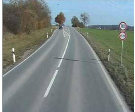
The limitation of the maximum permissible speed reduces the speed level at the intersection and increases the time gaps for turning into the major road.
