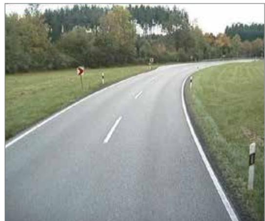
Individually placed bend chevrons indicate the direction of the bend.
